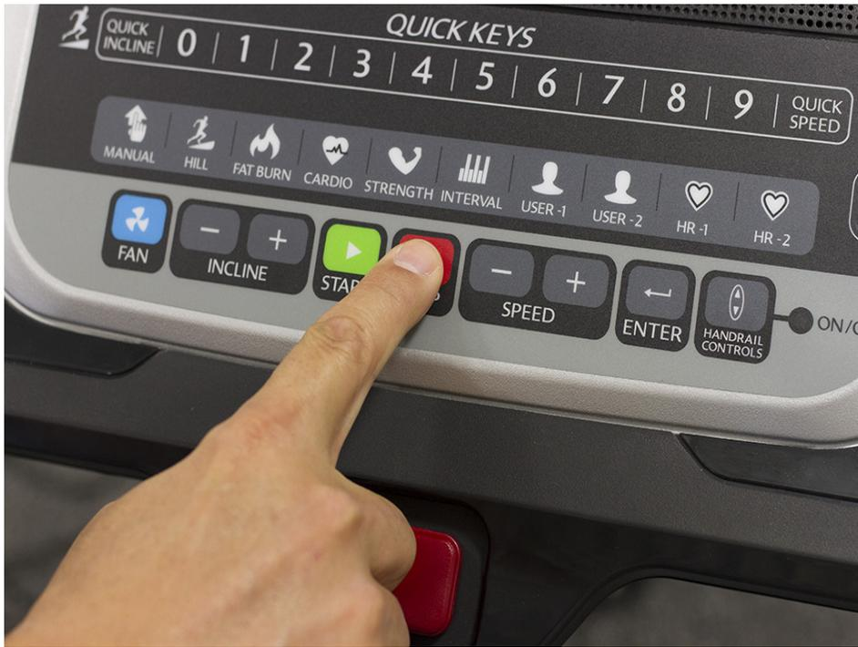
4. Once selection is made, press the STOP button to exit.
